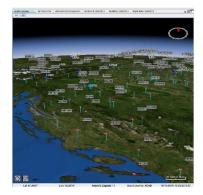
The Frequency Monitoring application provides 2D and 3D map windows to analyze the traffic situation from different perspectives. The maps can be use to overlay interrogation rate heatmaps, accumulated historical traffic and perform playback of recorded traffic. The system provides all data in raw and ASTERIX CATO21 format on network interfaces.
