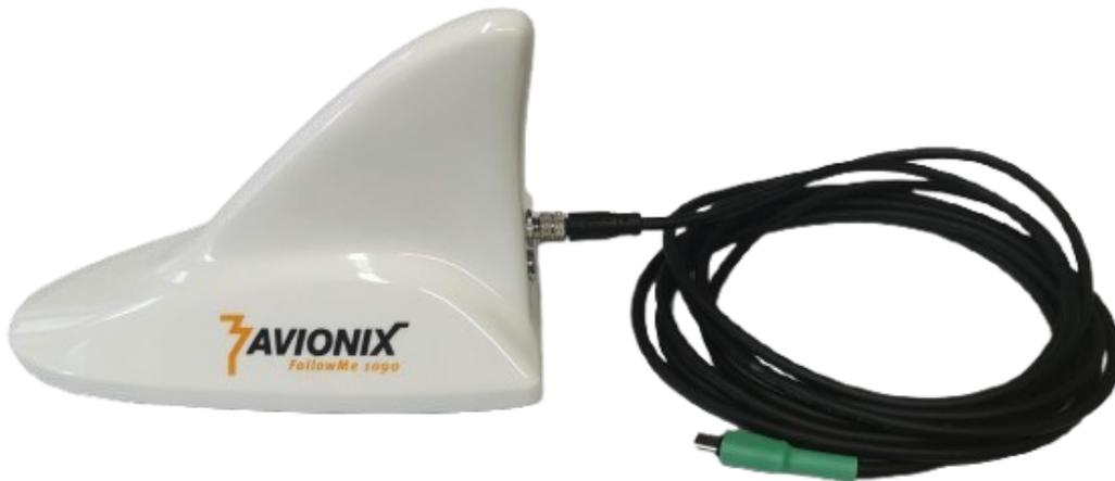
On the back side there is the 4 pin M8 connector and a dual colour red/green LED. The device is powered through the cable from 5-15V power input. A USB-A and a cigarette lighter adapter (9-32V) are provided to easily connect to various power sources.
